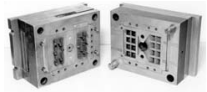
Figure 7. Laminated die made from steel sheets and the casting made in it (De Montfort University).
